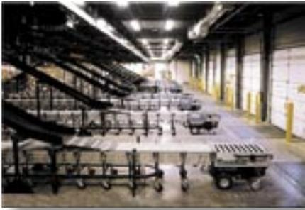
stop. When a carton reaches the discharge end of the conveyor it automatically stops. When the carton is removed from the conveyor bed, the conveyor starts again to bring the next carton into position.
